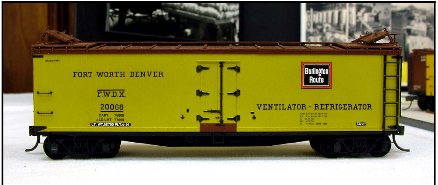
FWDX 20068, Accurail model upgraded with free-standing grab irons and ladders, A-Line sill steps (heated, straightened, and rebent to a more prototypical width and sharper corners), and Accurail Andrews trucks. The underframe has been modified to move the trucks nearer the ends of the car, and a scratchbuilt Murphy XLA roof replaced the kit's Hutchins roof. See Prototype Railroad Modeling Volume One for construction details of this model.
