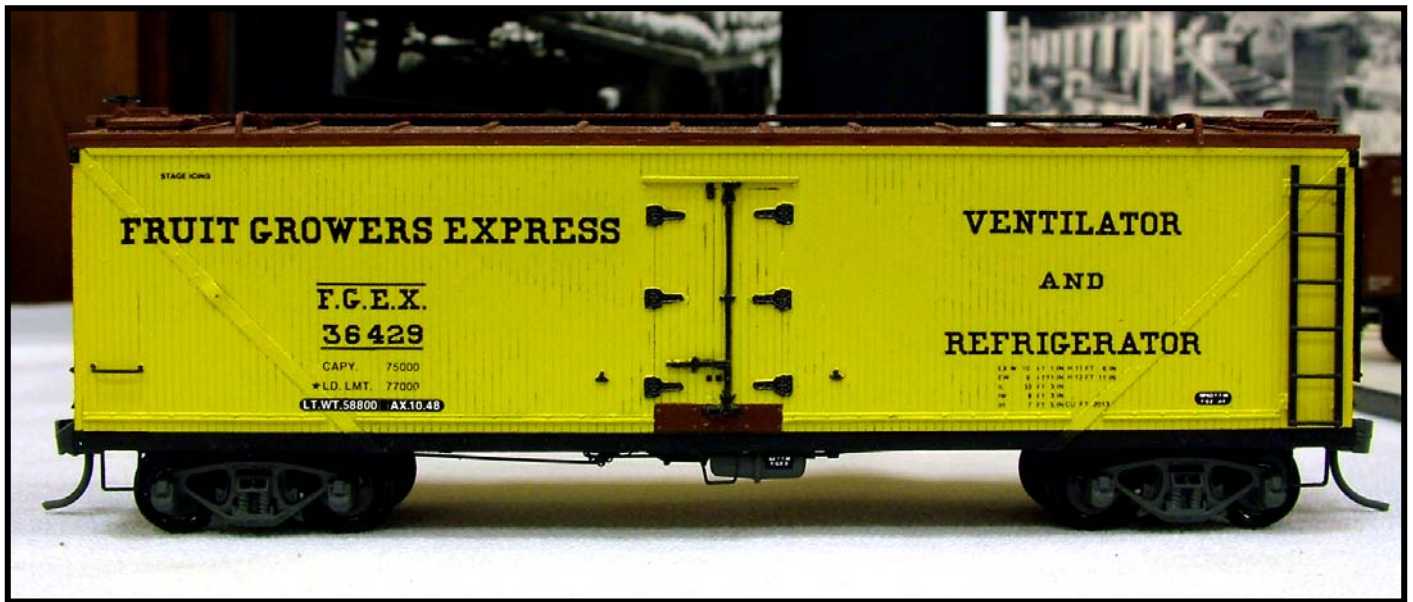
FGEX 36429, model built from Sunshine Models kit #34.2 and modified with diagonal sheathing straps.
